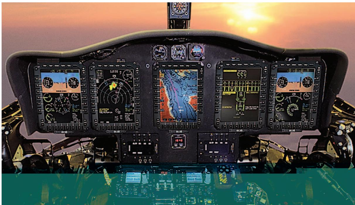
*The S-92 cockpit and display panel, shown here with an optional fifth liquid crystal multi-function display.*
