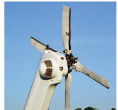
*Anti-torque control is provided by unlimited life tail rotor blades with bearingless composite flexbeam. Pitch control links use elastomeric bearings.*
