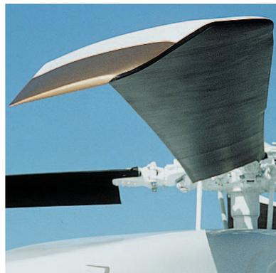
*Unlimited life main rotor blades incorporate composite spar technology and utilize a swept, tapered anhedral tip. This design provides improved lift and maneuverability.*
