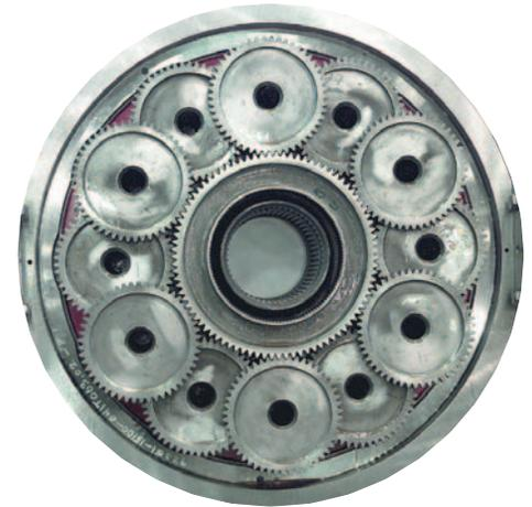
*The S-92 main transmission features a unique planetary gear system, and utilizes advanced materials for long life.*
