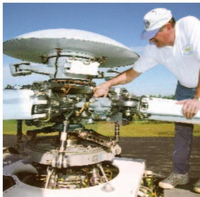
*The flaw-tolerant hub and yoke design provides unlimited life and improved safety, and the main gearbox incorporates advanced corrosion-resistant materials and coatings.*
