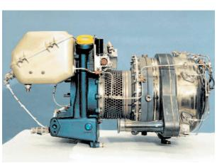
APU provides ground power and engine start, and is flight rated for emergency/supplemental power.
