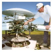
The flaw-tolerant hub and yoke design provides unlimited life and improved safety, and the main gearbox incorporates advanced corrosion-resistant materials and coatings.
