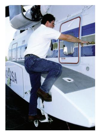
Built-in work platforms, hand- and footholds and walkways.
