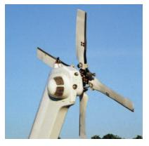
Anti-torque control is provided by unlimited life tail rotor blades with bearingless composite flexbeam. Pitch control links use elastomeric bearings.
