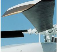
Unlimited life main rotor blades incorporate composite spar technology and utilize a swept, tapered anhedral tip. This design provides improved lift and maneuverability.
