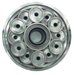
The S-92 main transmission features a unique planetary gear system, and utilizes advanced materials for long life.
